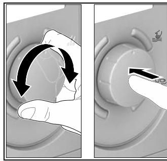
Turning and then pressing the rotary selector switch allows you to set the selected water temperature and use the menu (see chapter "Using the menu").
